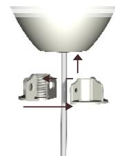
Put the two matching bottom parts together, facing each other, around the cord between the cover and the lamp. Insert the assembled bottom part into the cover by fitting the "wings" into the slots inside the cover. Push it into the cover until fully seated.
