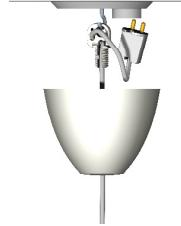
Hang the screw on the ceiling hook and connect the plug. (or terminal block). First ensure that the ceiling hook is fixed to the ceiling and does not rotate. When connected, collect the remaining cord, wind it around the upper part of the screw and hook and tie it up using the enclosed wire-tie (avoid winding it around the thread).
