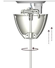
Move the lamptop upwards towards the screw hanging on the hook. When the screw and the bottom parts' "nut" have come in contact inside the cover, start screwing the cover clockwise until it reaches the ceiling. By pulling the cord lightly from below, the screw will automatically be angled downwards and will then easily find the nut.
