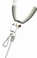
Insert the screw, plug and remaining cord through the cover from below. Also insert it through the ring if this is to be used. The ring can be used to make the cover bigger, or if the outlet for the ceiling lamp is located at a distance from where the lamp is to be placed. Push out a perforated tab to make room for the cord and place the ring to the ceiling on top of the cover.
