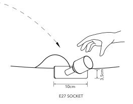
$\ensuremath{\mathsf{STEP 1}}$  The socket is mounted on a small magnetic plate.
