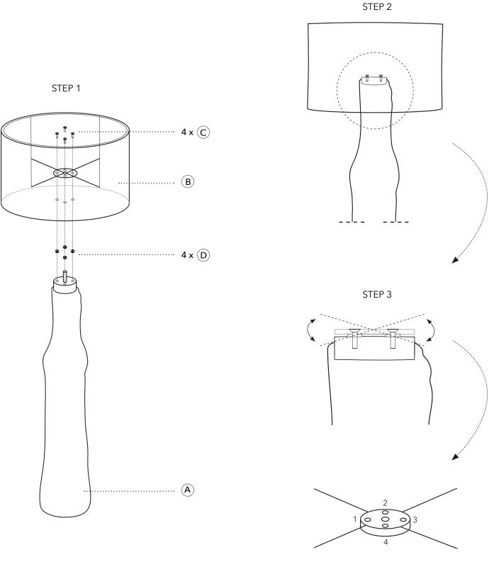
Use screw 1, 2, 3, 4 to adjust the position of the lampshade to reach perfect stability and horizontal alignment.
